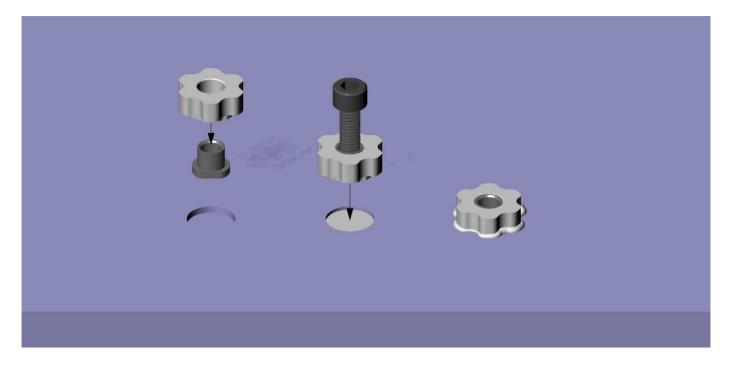
Semi-recessed Squirrel® Fixings have been developed to allow fabricators to make a mechanical screw fixing onto a 6mm sheet of solid surface material. The insert is recessed to a maximum of 2mm into the back of the sheet to prevent it from being visible through the face side. Please note that the inserts will be visible through translucent colours.
